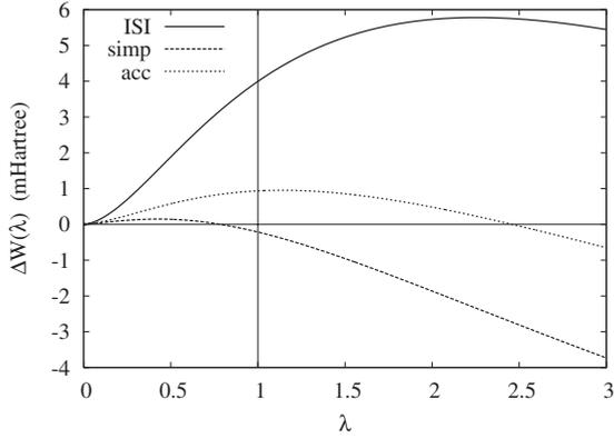
FIG. 1. Comparison of three different approximations to  $W(\lambda)$  for Hooke's atom ( $k=1/4$ ), plotted as  $\Delta W = W^{\text{model}} - W^{\text{exact}}$ . The exact curve (up to  $\lambda=3$ ) is taken from Ref. [19].
