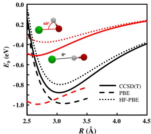
FIG. 4 (color online). Potential energy surface scans for the  $\text{HO} \cdot \text{Cl}^-$  complex along  $\text{Cl}-\text{O}-\text{H}$  angle of  $0^\circ$  (hydrogen-bonding structure, black lines) and  $60^\circ$  [hemibonding structure, gray (red) lines] using various methods;  $R$  is the  $\text{Cl}-\text{O}$  separation.
