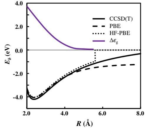
FIG. 3 (color online). Energy of NaCl as a function of Na-Cl distance in several calculations, and the PBE HOMO-LUMO gap.
