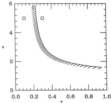
FIG. 5. Plot of constant error,  $\Delta=0.1$ , for the EBA in the semiclassical regime,  $\kappa \rightarrow \infty$  (actually,  $\kappa=31.83$ ). The EBA (and thus the TA) works to the left of and beneath this curve. The squares represent the  $\kappa \rightarrow \infty$  limit of the two curves plotted in Fig. 4.
